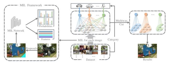
Fig. 2. An overview of the proposed method. The training images with image-level labels are used to train our MIL-based multi-label image classification network, as in Section 4. All training images, together with corresponding proposals, are fed into the MIL network to calculate the probability distributions and semantic features. A large knowledge graph is then constructed using all training images. The pseudo instance segmentation can be obtained using an improved multi-way cut algorithm.
